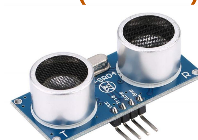
Ultrasonic Range Sensor (HC-SR04)
